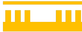
Fig. 1. Drawing of the groove waveguide and metal lid above it.
