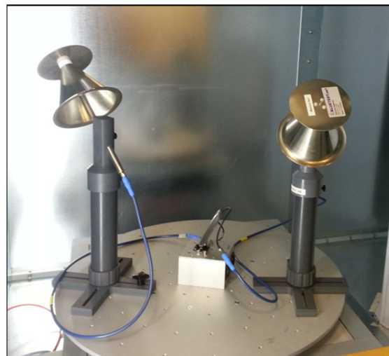
Figure 1.3. A photo showing LTE USB modem connected to two external antennas inside reverberation chamber during OTA MIMO LTE throughput measurements.
