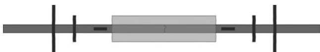
Figure 1. Schematic of the location marks, placed on both sides of a grain boundary, which is covered by a protective Pt strip.
