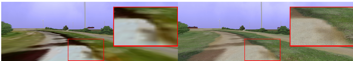
Figure 18. The figure shows that the color-coded image technique (right) enhanced the visual quality compared with only using aerial photos (left).
