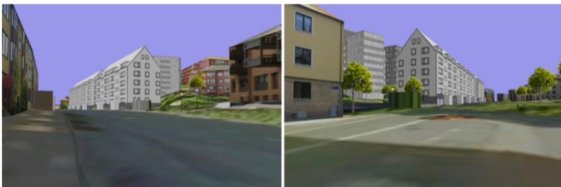
Figure 15. Snapshot from a VR model that was used to study proposed new buildings at Danskavägen, Gothenburg, Sweden. This VR model is a good example of how the technology can be used cost efficiently. This model was made in less than one day by using MrViz. This was made in-house by the city planning authorities in Göteborg using drawings from the building permit for the new buildings. The VR model was used by the neighbours and politicians to investigate how the new buildings would affect the views of the city from nearby apartments. The result from this line of sight analysis was that the different stakeholders came to a positive consensus regarding the project.
