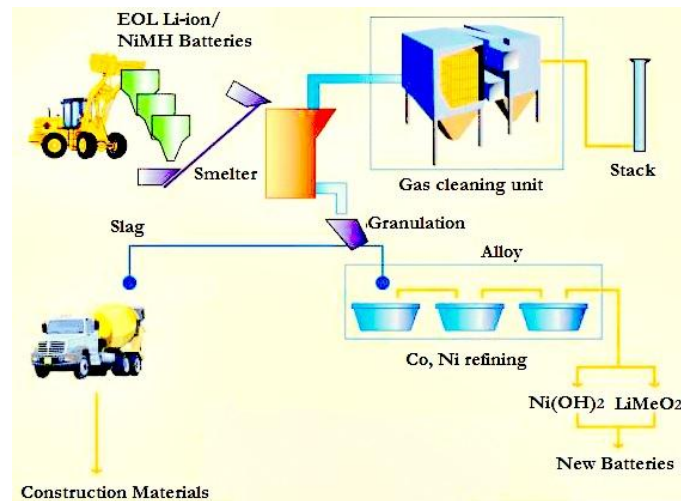
Figure 22: Umicore's, Val'Eas closed-loop process for recycling Li-ion batteries, (Bernardes, Espinosa et al. 2004)
