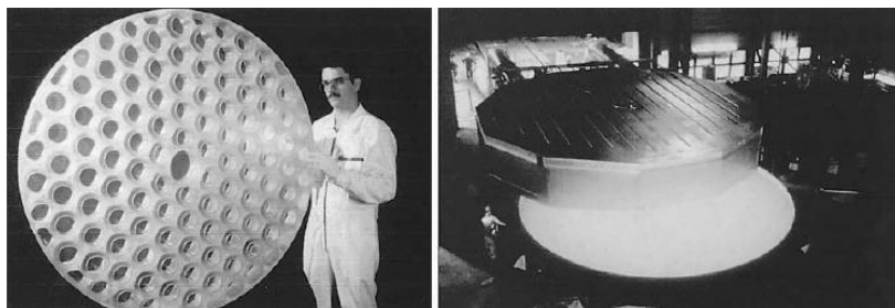
Figure 14: Examples of glass ceramics for telescopes; left, support; right, 8.6 m dia mirror (Garrett 2004)
