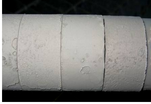
Fig. 6.4b. Deposits on the corrosion probe rings after four weeks' exposure with normal fuel mix and injection of ammonium sulphate (test case AS).
