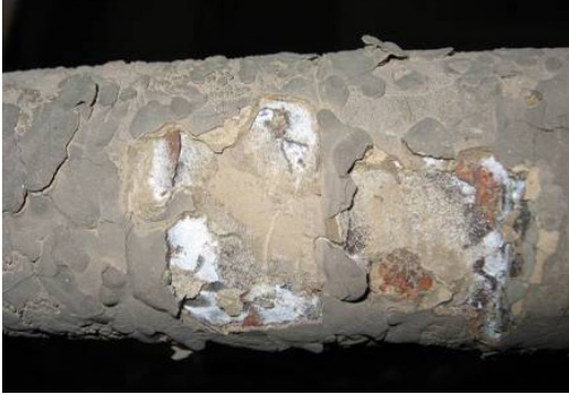
Fig. 6.4a. Deposits on the corrosion probe rings after four weeks' exposure with normal fuel mix (test case Ref).
