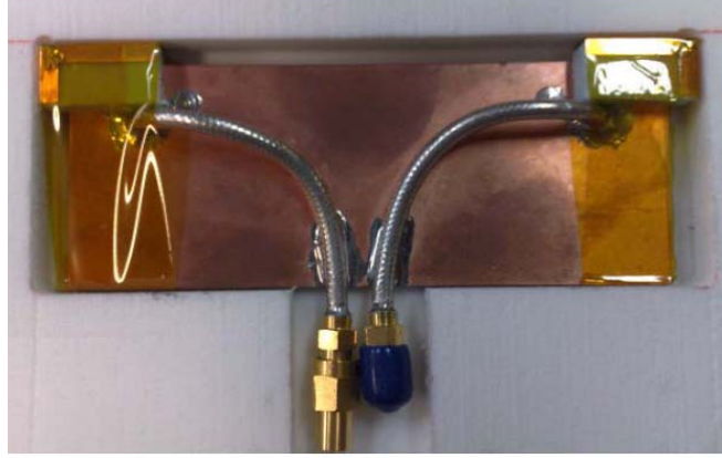
Figure 3.17: Photo of the two-port portable antenna used for verifying S-parameter method.
