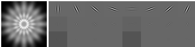
Fig. 2. A bank of Gabor wavelets in (a) frequency domain and (b) real parts in spatial domain.
