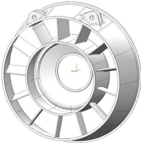
FIGURE 5: Turbine structure CAD model
