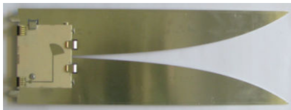
Figure 2: Single Vivaldi antenna element used in EMBRACE.
