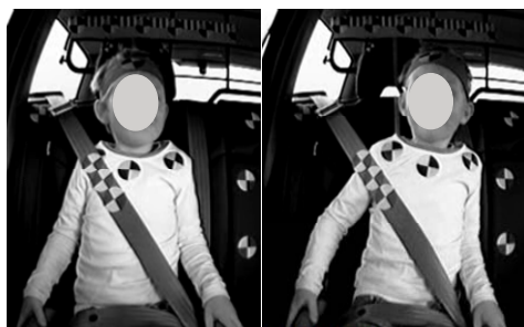
Figure 6. Sitting posture before and during the swerving maneuver in the study by Bohman et al. 2011
