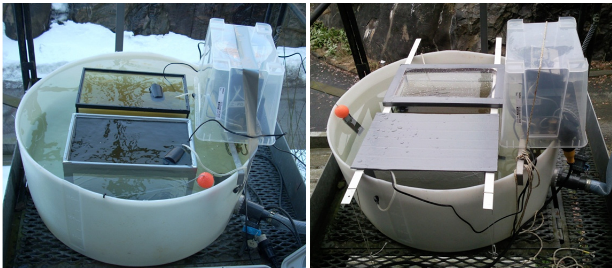
Figure 3 Microcosm experiment arrangement, left – microcosms without lids, right – the same microcosms covered with lids.
