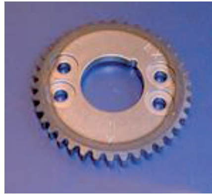
Timing sprocket for automotive engine.
