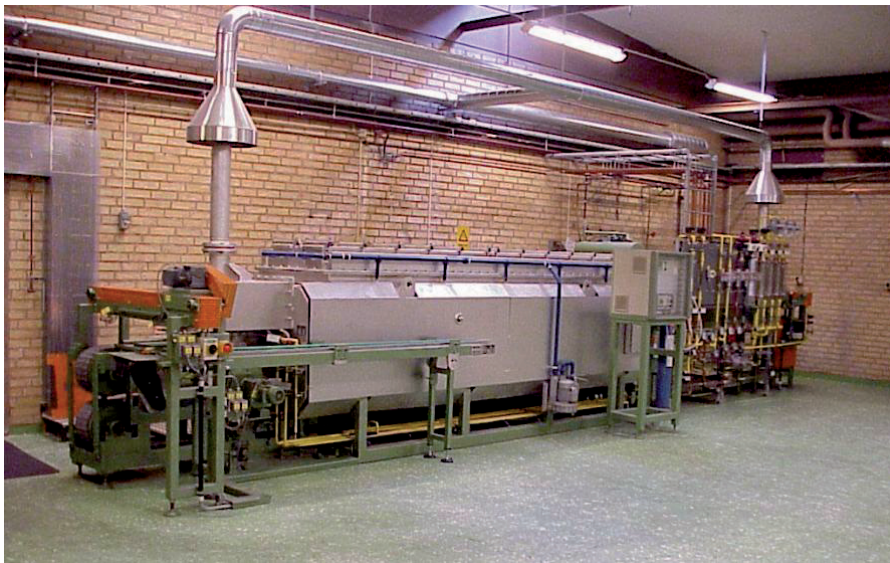
Figure 17. Laboratory mesh belt furnace used for sintering trials in the research studies described in Paper II and Paper IV.
