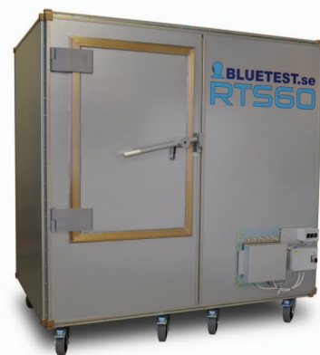
Figure 1. Photo of a Bluetest reverberation test system RTS60 used in the presented measurements. Cavity size of the chamber is 1.75m x 1.8m x 1.2m.
