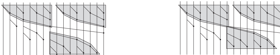
Fig. 16. Even when a network uses fanout greater than two, it will have a left-hand part that uses only fanout two, or possibly one fanout of three at the waist. The arrangement on the left (which shows only part of the network working on an initial subsequence of the inputs) shows how the resultant binary trees of operators are arranged for odd depth. For even depth, we squeeze one of the trees up against the waist. In either case, the top partition will contain at least k 2s, where k = 2^{\lfloor d/2 \rfloor} , for depth d . The concrete trees shown here are of depth 3, but a similar pattern applies for deeper trees.
