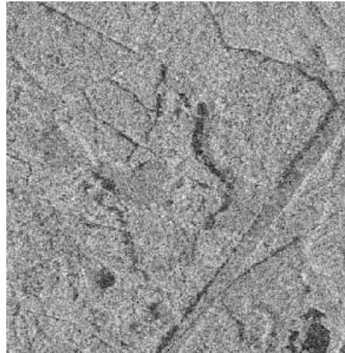
Fig. 4a. Radarsat-2 UltraFine HH polarized image (look angle \sim 41^\circ ) acquired on 2009-08-23 before the simulated wind-throw.
