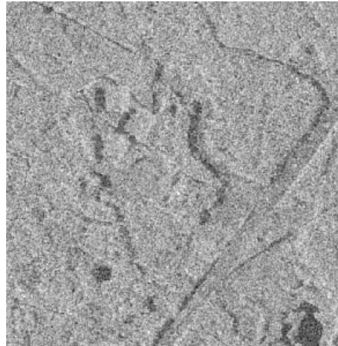
Fig. 4b. Radarsat-2 UltraFine HH polarized image (look angle \sim 41^\circ ) acquired on 2009-10-10 after the simulated wind-throw.
