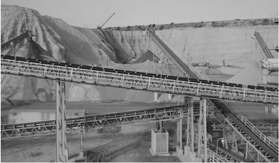
Figure 13. Conveyor belts are frequently used for transportation between different production units in crushing plants. VMC's Reliance operation, Irwindale, CA, USA.
