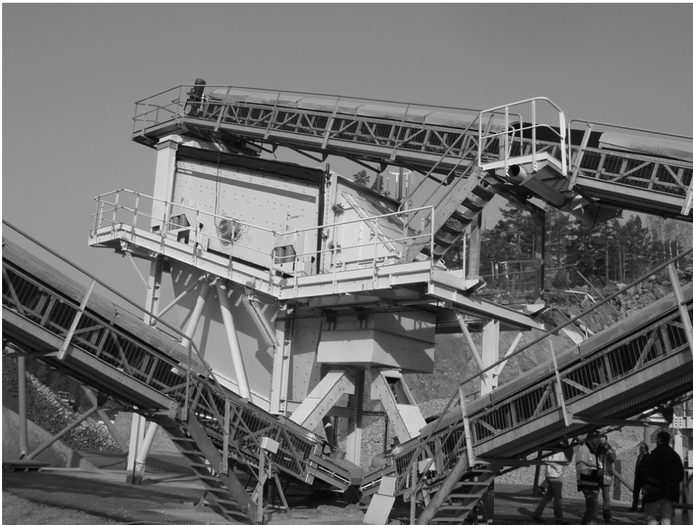
Figure 12. This screen is fed from the conveyor on top coming in from the right. The products are conveyed on different conveyor belts away from the screen. NCC's Glimmingen operation, Uddevalla, Sweden
