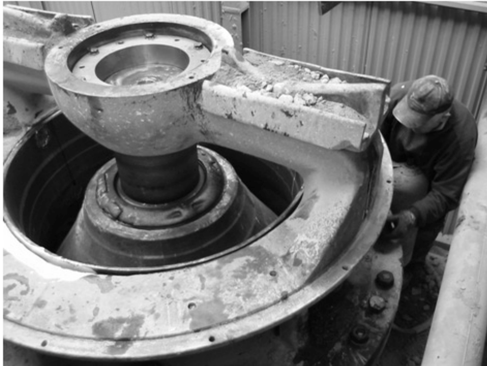
Figure 2. A Sandvik Hydrocone H6000 at NCC Roads' crushing plant Ramnslätt during assembly after a wear part change. The cone, main shaft and top bearing can be seen in the center of the crusher.
