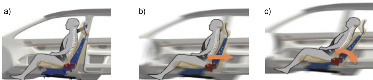
Figure 20. Whiplash Protection System (WhiPS). a) Normal position b) Translational motion c) Reclining motion. Reprinted with permission by Ola Boström, Autoliv.
