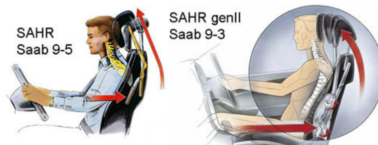
Figure 19. The Saab Active Head Restraint (SAHR) generation I (to the left) and generation II (to the right). Reprinted with permission by Stefan Olsen, Saab.
