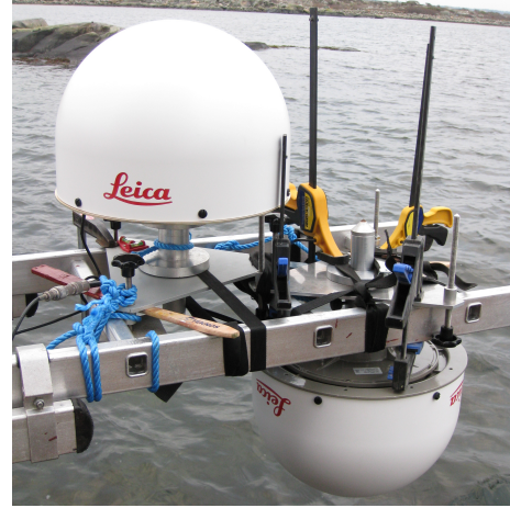
Figure 2. The experimental setup of the GNSS-based tide gauge at Onsala Space Observatory.
