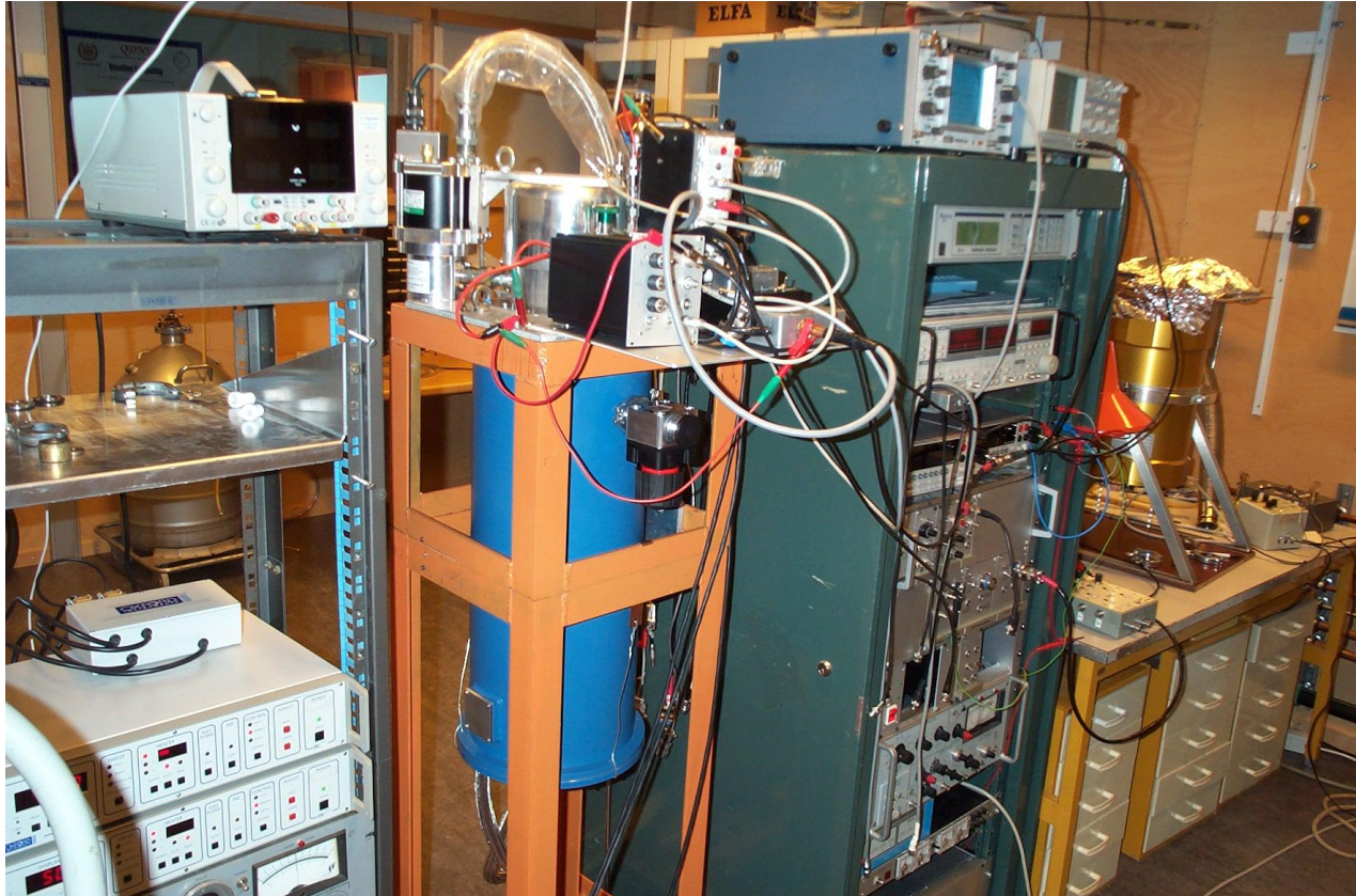
Figure 8. View of the experimental setup with HELIOX AC-V in the center and conventional INFRARAD Labs cryostat to the right.
