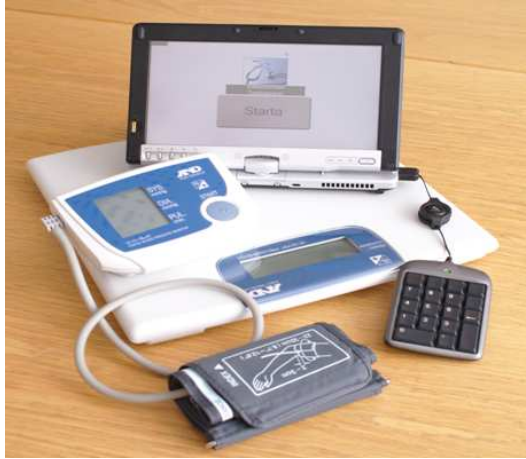
Figure 3.15: Photograph of the first home terminal prototype, including the medical equipment, tablet PC and numeric keyboard.
