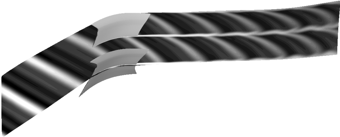
Fig. 3 Entropy contours at a mid-radius-surface and blades, over the two stator passages used in the wake response computation. Wakes are entering from the left through the unsteady inflow b.c. and seen as light strikes that are convected downstream (to the right) with the flow.
