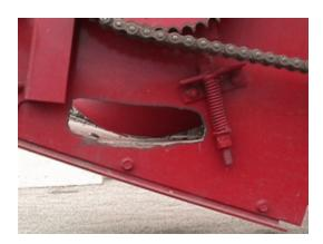
A hole is cut in one end of the header to blow grain out. Operators simply take an air hose, start in the far end and blow grain across the table and out the exit hole. It is difficult to blow the grain out of a header without the hole because wind in the corner catches kernels deflecting them back into the header. Vacuuming is difficult because it is difficult to reach completely around the auger.
