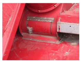
Adding a door to the sump of the vertical auger facilitates access and clean out. Note that this operator also added a small wood filler near the base of the sump to prevent kernels from falling into the tight bottom crevice.
