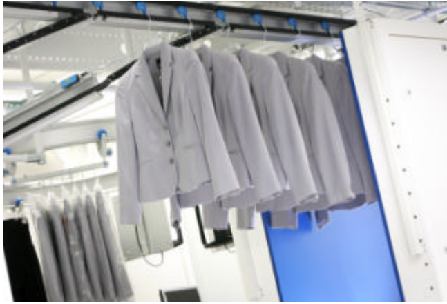
Figure 27: Hanger Goods Sorter. Source: Metro Group
