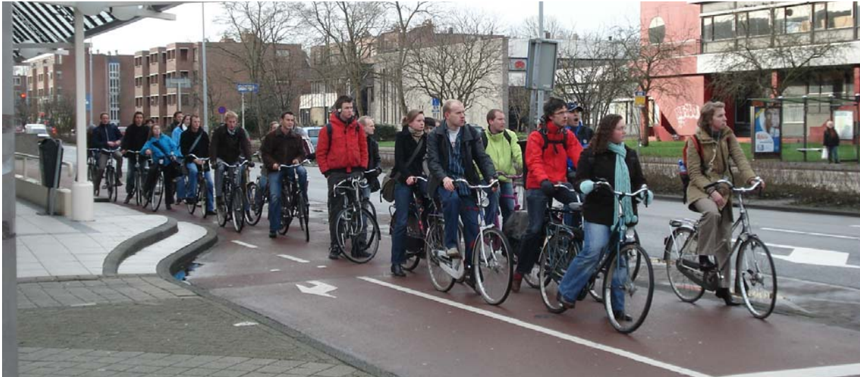
Figure 1.1: Approximately 20 bicyclists at a traffic light take up less space than three or four small cars.
