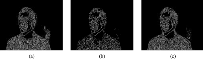
Fig. 5. Generating interior moving Canny edges by the two methods. (a) Original interior Canny edges. (b) Interior moving Canny edges obtained by the two-frame-based method. (c) Interior moving Canny edges obtained by our multiframe-based method.
