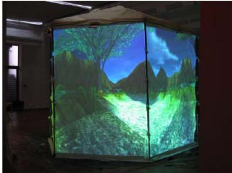
Fig. 3. Simple CAVE generated with canvases fastened on hexagonal scaffolding
