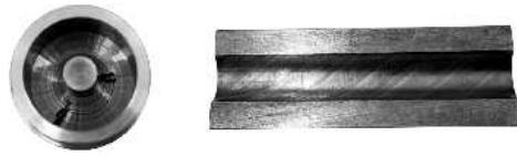
Figure 2: Radial chatter marks on the bottom of the bore hole (left) and effects of spiralling on the bore hole wall (right).
