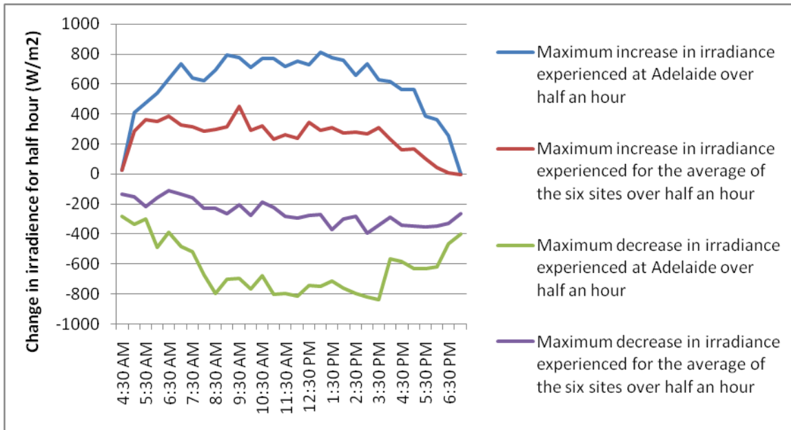
Figure 6: Maximum irradiance changes for time intervals for Adelaide and for the average of the six sites.
