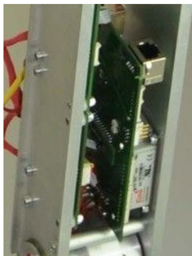
Figure 4-6: Aluminum skeleton chassis used to convey the heat away from the controller
