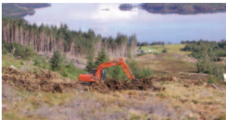
◉ United Kingdom Photo 18.2 | Excavator cultivation on an upland restock site to improve tree establishment and suppress weed vegetation (Forestry Commission/Alistair Macloed).
