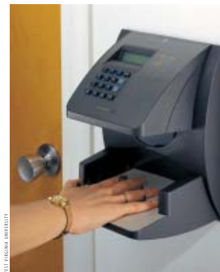
Biometric technologies like this hand reader identify individuals by their physical characteristics.
