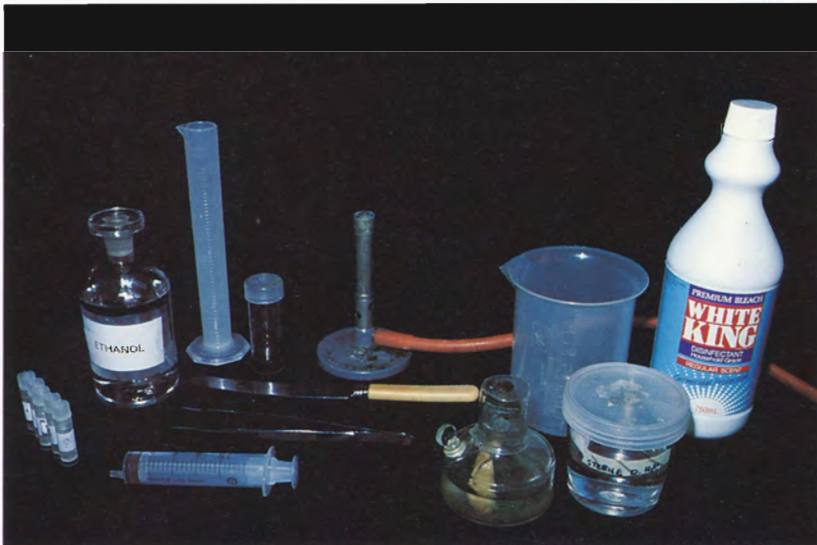
Figure 5. Equipment required for isolation and surface sterilisation of the embryo.
