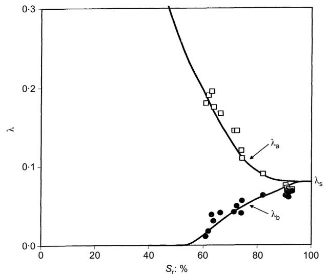
**Fig. 13. Variation of critical-state compressibilities with degree of saturation for Jurong soil [ $v = \Gamma_{ab} - \lambda_a \ln(p - u_a) - \lambda_b \ln(u_a - u_w)$ ]**
