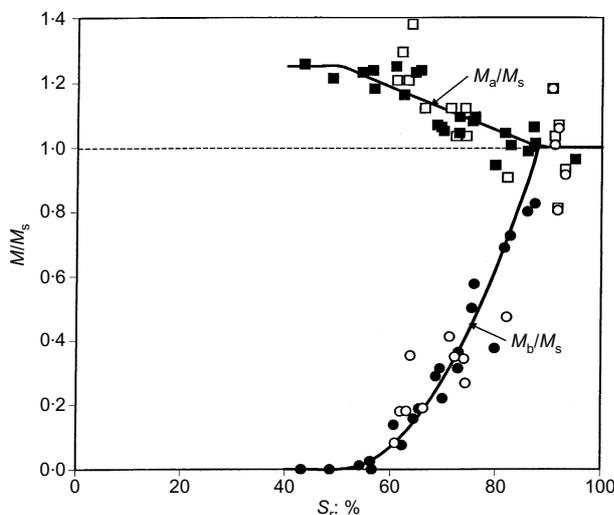
**Fig. 12. Normalised functions for critical-state stress ratios (solid symbols, Kiunyu gravel; open symbols, Jurong soil)**
