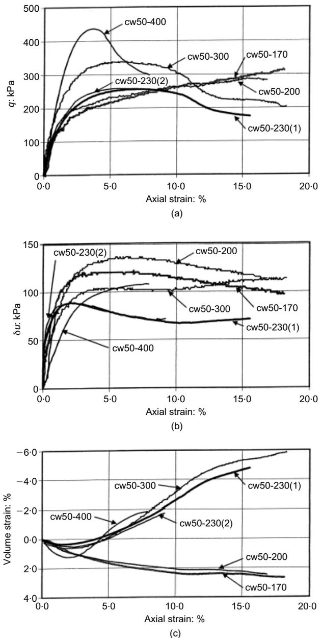
**Fig. 5. Results for constant water content tests at net confining stress of 50 kPa and various matric suctions, plotted against axial strain: (a) deviator stress,  $q$ ; (b) change in pore water pressure,  $\Delta u$ ; (c) volume strain**
