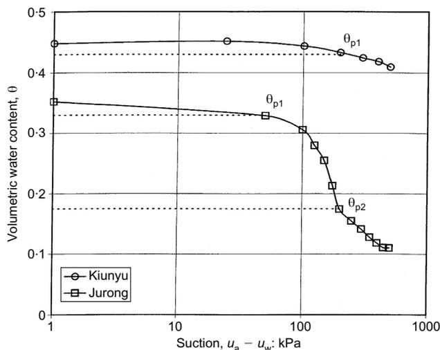
Fig. 17. Soil-water characteristic curves for Kiunyu gravel and Jurong soil
