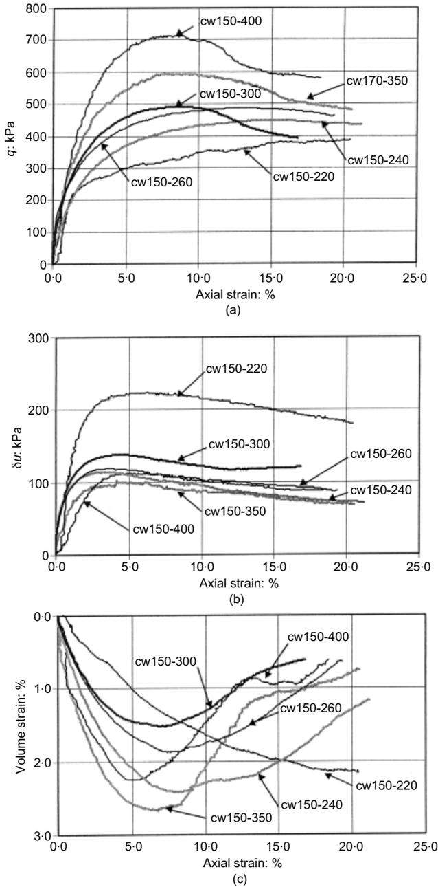
Fig. 6. Results for constant water content tests at net confining stress of 150 kPa and various matric suctions, plotted against axial strain: (a) deviator stress,  $q$ ; (b) change in pore water pressure,  $\Delta u$ ; (c) volume strain
