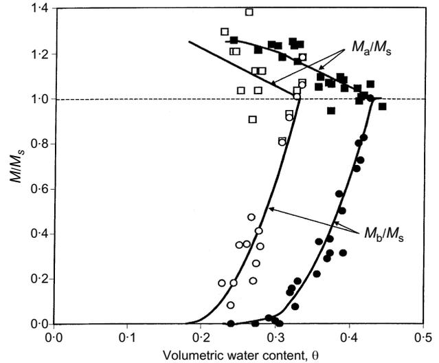
Fig. 15. Variation of critical-state stress ratios with volumetric water content (solid symbols, Kiunyu gravel; open symbols, Jurong soil)
