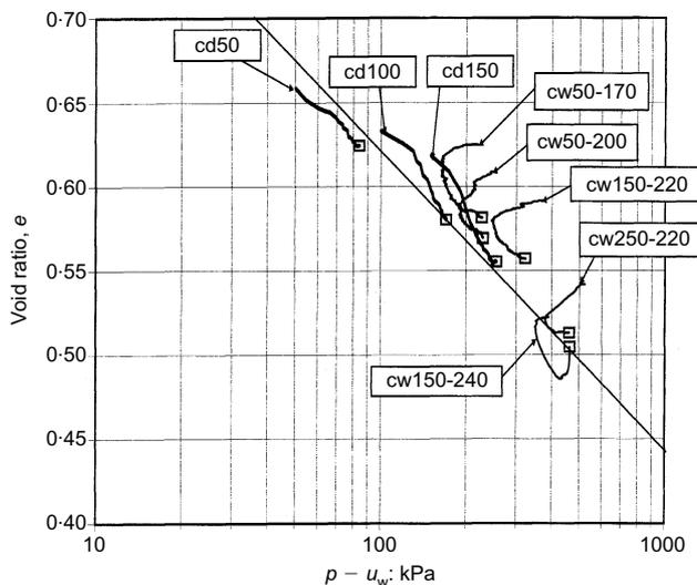
Fig. 10. Void ratio,  $e$ , plotted against  $p'$  for saturated drained tests and constant water content tests at high degrees of saturation
