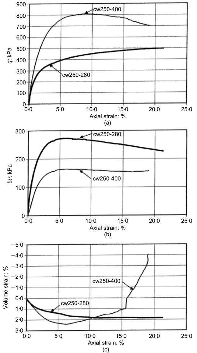
Fig. 7. Results for constant water content tests at net confining stress of 250 kPa and various matric suctions, plotted against axial strain: (a) deviator stress,  $q$ ; (b) change in pore water pressure,  $\Delta u$ ; (c) volume strain
