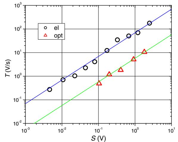
FIG. 3 (color online). Dependency of the rise of the transient triplet absorption signal ( $T$ ) on its corresponding fluorescence level ( $S$ ) for electrical and optical excitation on a double logarithmical scale. The two solid lines are least-squares fits of the offset of a strictly linear dependency.
