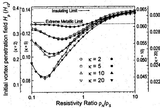
FIG. 4. Initial vortex penetration field  $H_p$  as a function of  $\rho_N/\rho_S$  for  $\kappa=2, 5, 10$ , and  $20$  for rectangular (open symbols) and circular (closed symbols) superconductors. The y-axes are scaled so that the asymptotic values of  $H_p$  in both the insulating and extreme metallic limits are at the same position for all  $\kappa$  values.
