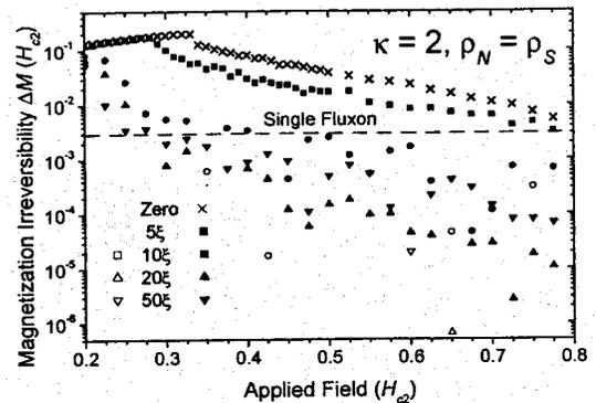
FIG. 9. Magnetization irreversibility on a logarithmic scale for  $\kappa=2$  superconductors with  $\rho_N = \rho_S$  normal metal coatings and  $S'$  layers of various thicknesses. (Negative values are indicated by open symbols.)
