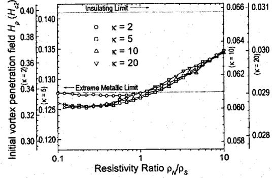
FIG. 5. Initial vortex penetration field  $H_p$  as a function of  $\rho_N/\rho_S$  for  $\kappa=2, 5, 10$ , and  $20$  for rectangular superconductors where  $T_{c(N)}=-2T_{c(S)}$ . The y-axes are scaled so that the asymptotic values of  $H_p$  in both the insulating and extreme metallic limits are at the same position for all  $\kappa$  values.
