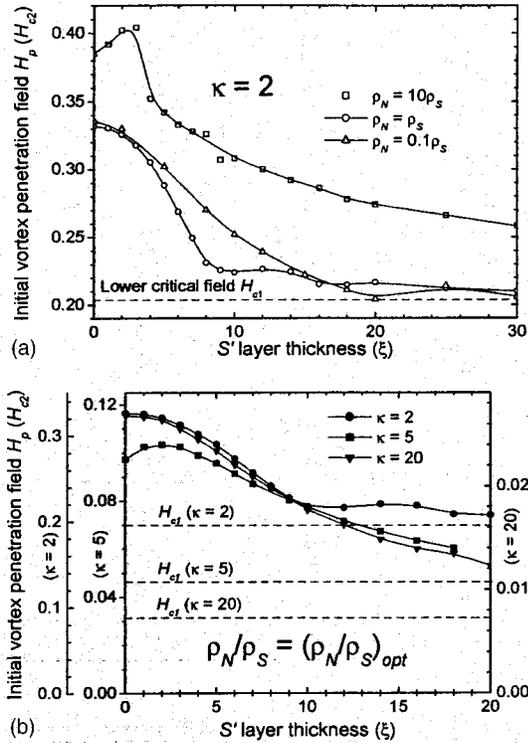
FIG. 10. Initial vortex penetration field  $H_p$  as function of  $S'$  thickness for (a)  $\kappa=2$  superconductors with  $\rho_N=\rho_S$  and  $\rho_N=10\rho_S$  normal metal coatings, and (b)  $\kappa=2, 5,$  and  $20$  superconductors with coating resistivity given by  $(\rho_N/\rho_S)_{opt}$ . The y axes are normalized to  $H_p$  for a  $10\xi$ -thick  $S'$  layer.
