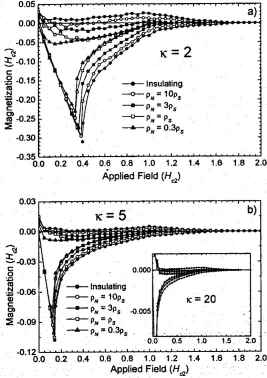
FIG. 3. Magnetization of a superconductor with an insulating surface and of superconductors with normal metal coatings of various resistivities (a)  $\kappa=2$ , (b)  $\kappa=5$  with an inset for  $\kappa=20$ .
