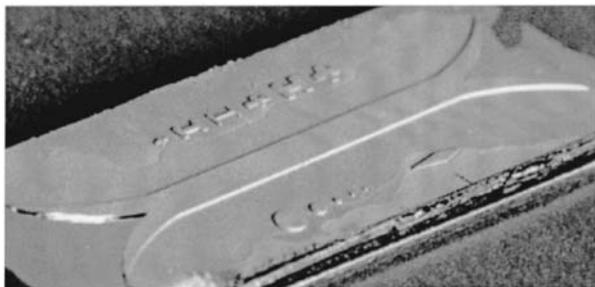
Fig. 3. Photograph of micromachined waveguide with antennas at both ends.
