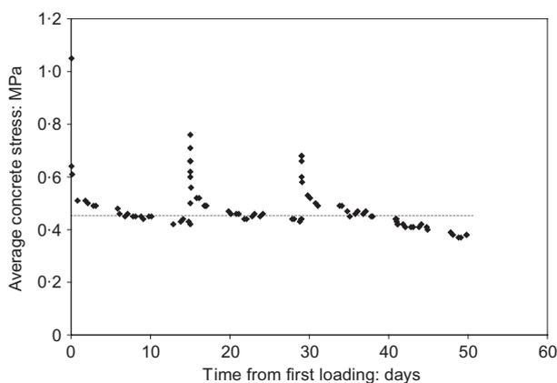
Fig. 14. Variation in concrete stress with time for specimen T16R2
