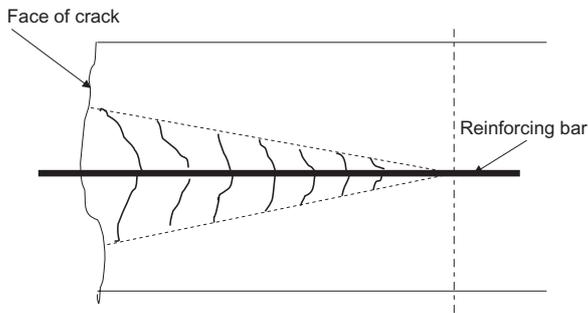
Fig. 2. Internal cracks as established by Goto<sup>6</sup> and Otsuka and Osaka<sup>7</sup>
