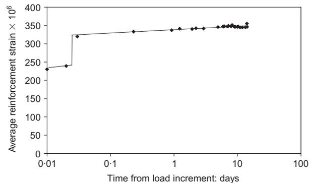
Fig. 4. Specimen T20R3—change in strain under load of 43 kN
