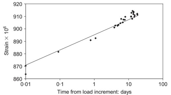
Fig. 8. Specimen T20R3—strain development under load of 71 kN
