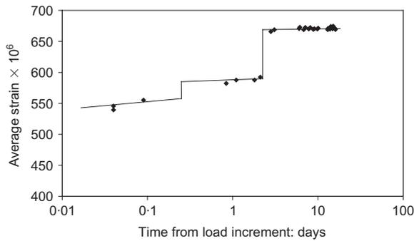
Fig. 5. Specimen T20R3—development of strain under load of 57 kN
