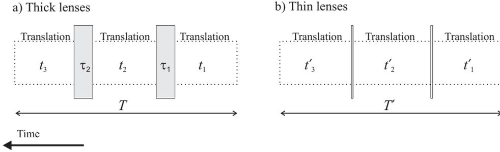
**Figure 2.** A schematic diagram showing the timing sequences for the two frames of reference. (a) shows the thick lens or lab frame with the time durations for each stage and (b) shows the mathematically equivalent thin lens representation that is used in the calculations. Note that the direction of time runs right to left so that it visually mirrors the system matrix layout in equation (5).
