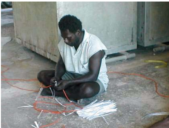
Figure A2.2 Attaching short pieces of raffia (tie-ties) to the main polypropylene line [above left]
