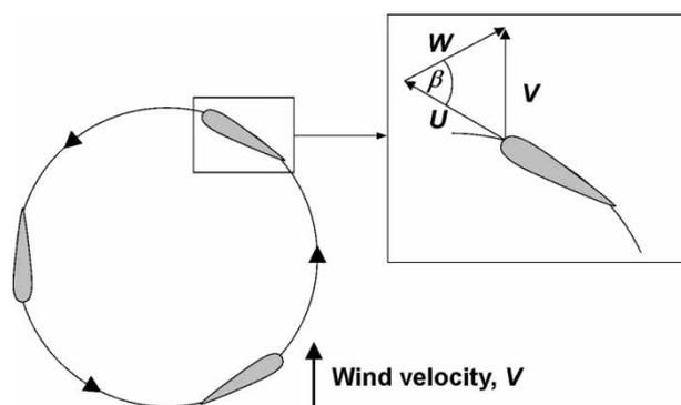
Fig. 1 Generic blade velocity triangle for a VAWT
