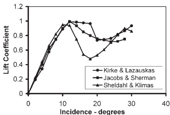
**Fig. 3** Comparison of published NACA 0012 lift coefficient data
