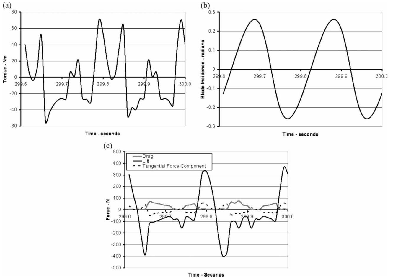
Fig. 7 Blade torque, incidence, and force changes during a single rotation: (a) rotor torque: single blade;  $3\pi/4$  starting position, (b) blade incidence: single blade;  $3\pi/4$  starting position, (c) blade forces: lift, drag, and net tangential component
