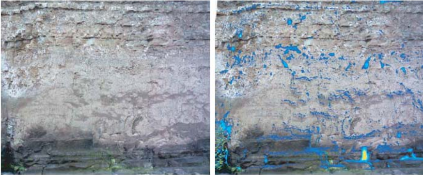
FIG. 6a: Site A: orthoimage and superimposed difference model (September 2003 – May 2004).
