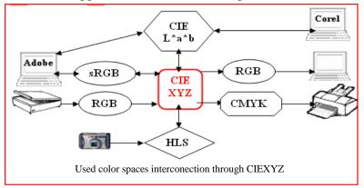
The ICC color profiles make the standard color corrections required for the color images transfer between PCS and the color spaces which depend on equipment or on the graphical application that were imposed as standards in the field (RGB, sRGB, CMYK). For creating ICC profiles pertaining to the equipments and programs of the technologic flow, specific programs and calibration devices are employed. CMM- ICC (or ICC compatible) achieves color transformations between source and destination spaces.
