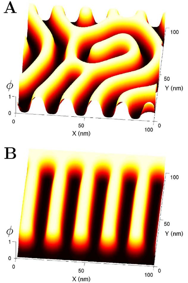
FIG. 2. (Color online) Diblock copolymer thin film morphologies showing (a) disordered and (b) ideal structures. The parameters governing the diblock copolymer are  $N=10\,000$ ,  $\chi=0.015$ ,  $b=0.24$  nm, and  $\alpha=0.001$ . The ideal morphology was created by introducing a range of interaction,  $r_0=3$  nm, at the surface and an electric field of  $E=3.5 \times 10^5$  V m<sup>-1</sup>. The dielectric constants of the donor and acceptor are 3 and 4, respectively.
