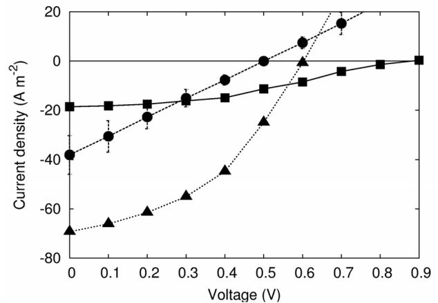
FIG. 4. Current-voltage ( $I$ - $V$ ) curves for systems with planar (■), disordered bulk heterojunction (●), and ideal (▲) morphologies.  $I_{sc}$  is defined as the current when  $V=0$  and, similarly,  $V_{oc}$  is defined as the applied voltage when  $I=0$ . The power conversion efficiency is given by the maximum value of  $I$ - $V$  divided by the total solar irradiance.
