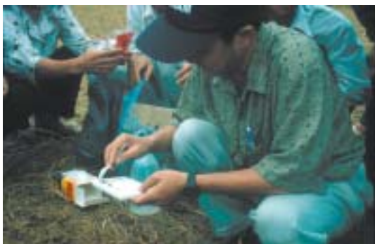
Figure 2.4 Measurement of soil pH in the field using either (a) a portable pH meter, or (b) a colorimetric soil pH test kit.
