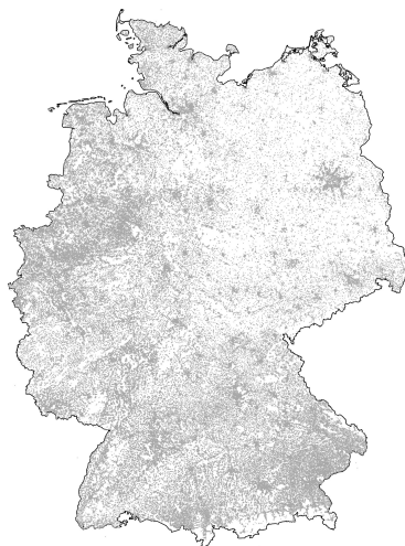
Figure 1: Distribution of PV systems within Germany until 2009; each gray dot points a PV system
