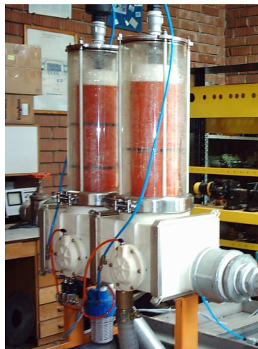
Figure 8. The modularized self flushing filter battery on test
