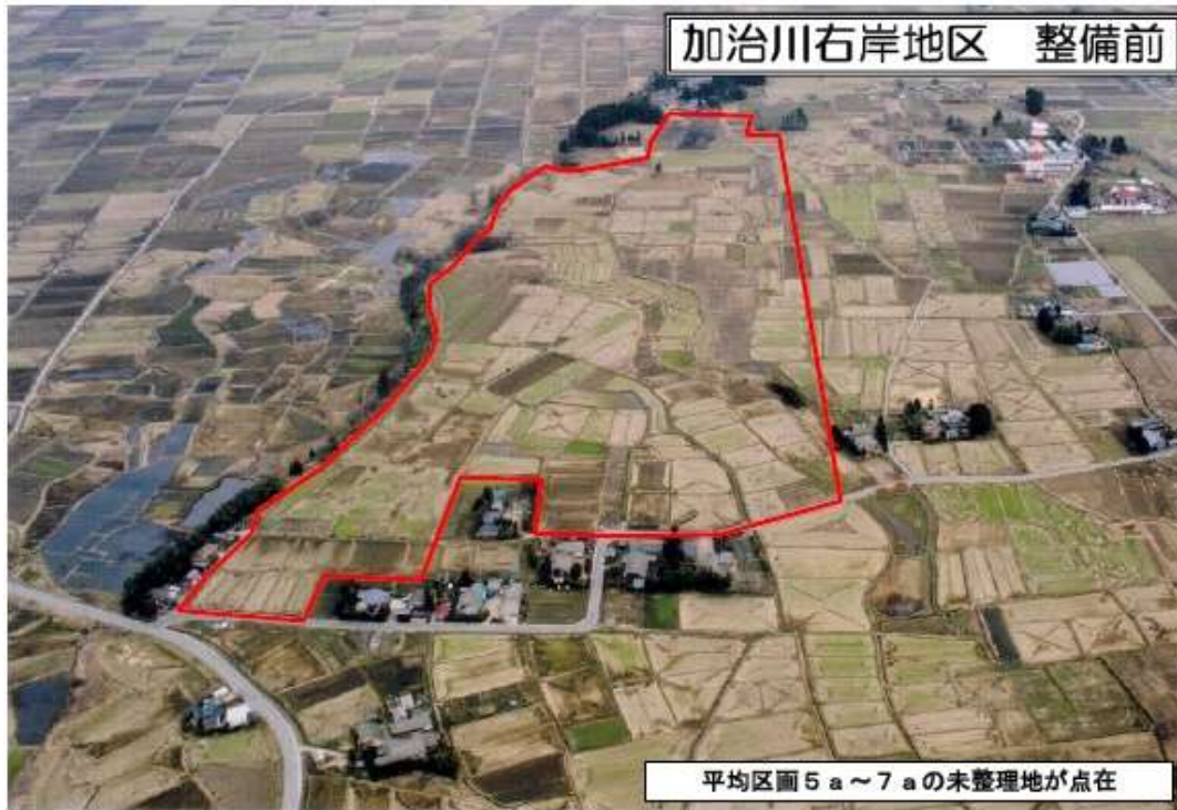
a) Before. Plots were in irregular shape and sizes were in average 0.05-0.07ha.
