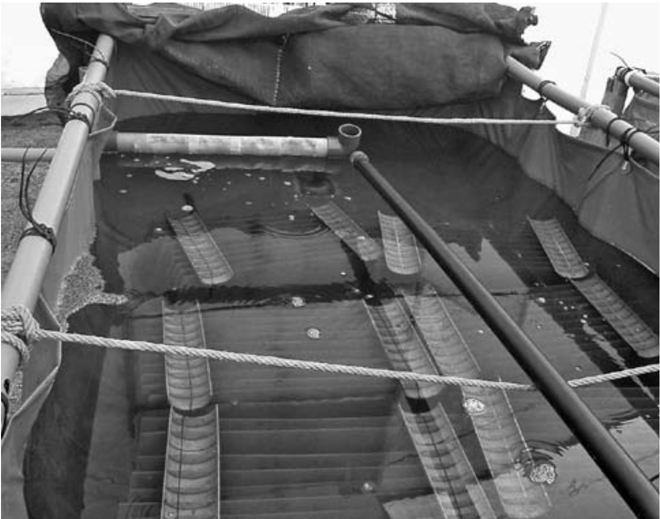
Figure 43. Nursery tank with settlement surfaces.
