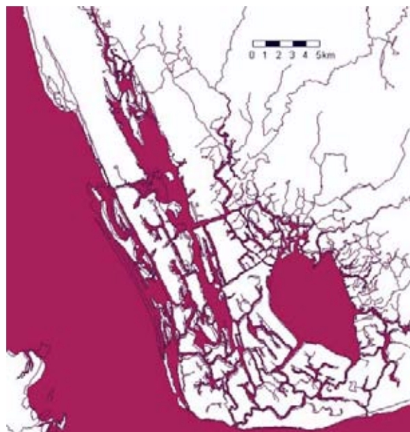
Figure 5: Complex network of channels as illustrated by Boeung Tonle Chhmar (upper central part of the Tonle Sap Lake). Blocking these channels would irreversibly change the hydrological, hydrodynamic and ecological functioning of the area. Source: Report "Influence of built structures of Tonle Sap hydrology and related parameters"
